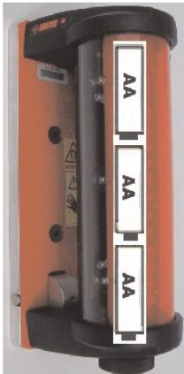
The receiver uses 3 AA alkaline batteries. Unscrew black cap at bottom of unit to replace batteries; orient as shown. Operating time is approximately 130 hours.
